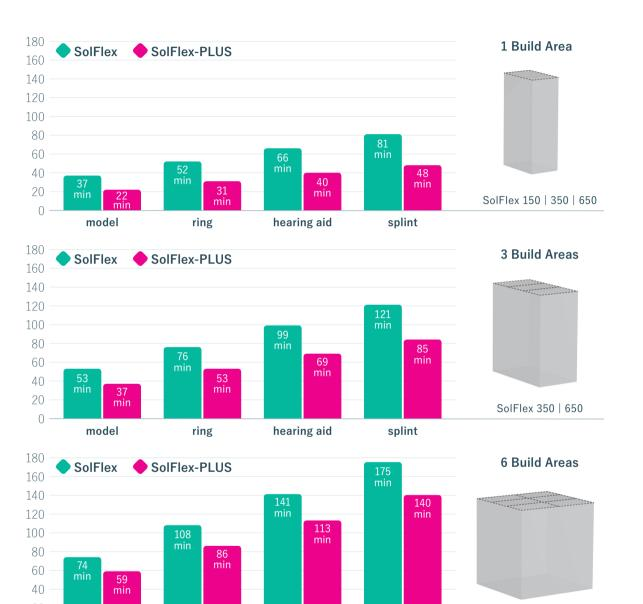
20 SolFlex 650 0 ring model hearing aid splint \$5cm/2.0in \$3cm/1.2in \$4cm/1.6in \$ 2 cm/0.8 in All stated times refer to parts 5 printed under the following conditions: Material: SolFlex Prototype Clear Light Intensity: 16mW/cm<sup>2</sup> Wavelength: 385nm BuildStyle: Normal
